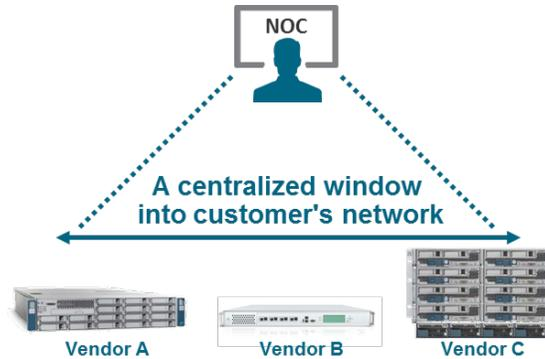
Open SNMP integrated in Ceragon's NMS enables discovery and management of SNMP-based equipment from other vendors
