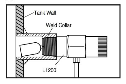
Operating Pressure: 2000 psi (13.8 MPa) [138 bar] Operating Temperature: 400°F (204°C)
