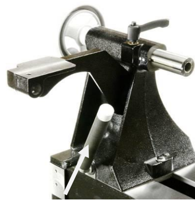
Tailstock clamp handle
