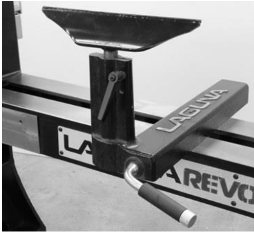
Tool rest assembled to the bed
