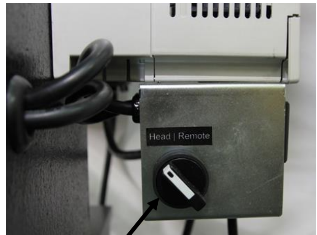
Controller selection switch
