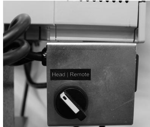
Head or remote selection switch
