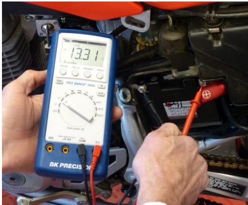
(above) Battery Voltage at idle.
