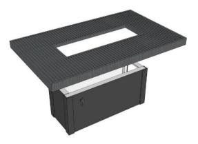
2. Place a bracket 12" from each corner on the long sides of the composite wood top and attach the brackets with the included sheet metal screws.
