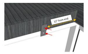
3. Before placing the concrete top, see the diagram below and mark out corner locations of the concrete with masking tape or a pencil.
