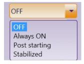
Always ON: FIFO recording of selected variables until the logger is Off.
