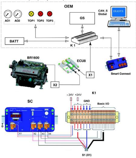
Via the K1 connection box, the ECU8, the Smart Connect and the module are connected: a CAN bus between the Smart Connect and the ECU8 with a proprietary protocol, a CAN bus between the Smart Connect and the module with the J1939 protocol. X4 is the connector supporting the J1939 to connect to the module.
