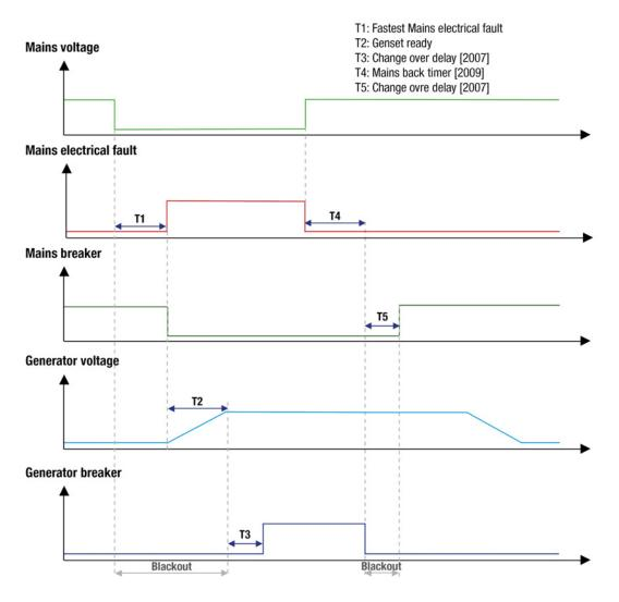
If a remote start is activated when the Mains is present, the Generator starts, opens the Mains breaker, closes the Generator breaker after a preset time and take the load.
