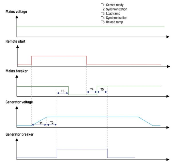
When remote start is off, the Mains takes the load in the same way as the Generator did previously. If the Generator started because of a Mains failure, when the Mains power returns the module synchronizes the load transfer (ramps down), opens the breaker and then stops the Generator as described below:
