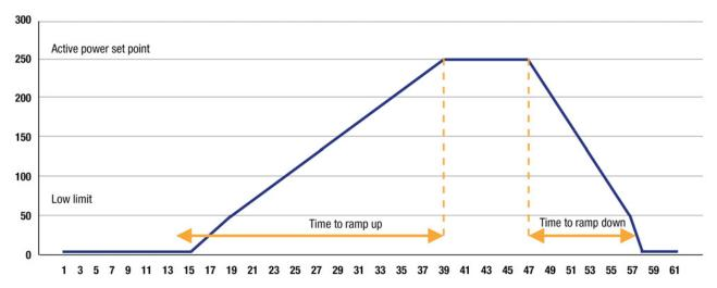
Before stopping the Generator, the module reduces its load to the low limit and then opens the circuit breaker. If the breaker opening fails at the end of the ramp, the Generator continues to share the load and shows a breaker opening fault on display.
