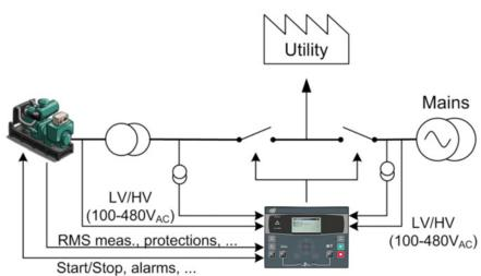
In change-over mode, the Generator starts and takes the load in case of a Mains failure.
