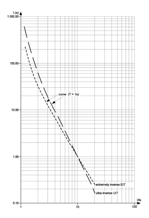
Inverse curves just above the pick-up value (not logarithmic abscissae I/Is) for various value of TMS:
