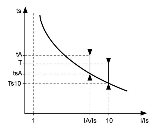
In the preceding curves in logarithmic plot, Ts10=1. For a given I/Is (first column of next table), find K in the row. Then  $ta = K \times T$ .
