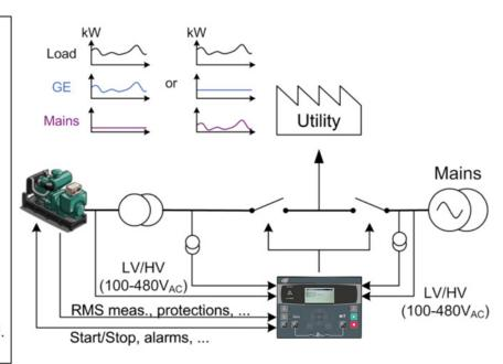
When the remote start is on, the module starts the Generator, synchronizes and parallels with the Mains, then ramps up load until it reaches its set-point.
