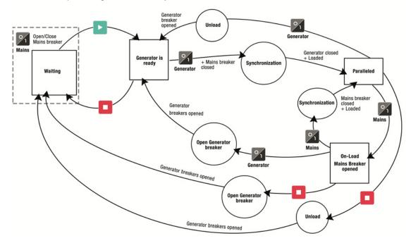
Note: MAN mode does not allow +/- fast or +/- voltage to synchronize or load control.
