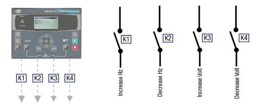
A digital potentiometer converting pulses into analog values can be used. A digital potentiometer has its own parameters:  $\Delta U0$  (fsd) and timer.
