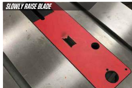
SLOWLY RAISE BLADE As the blade rises, the throatplate section will cut away. Stop the process at the desired blade height for application with the blade or dado set.
