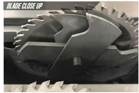
BLADE CLOSE UP Install dado set as shown to prevent chipper jamming.
