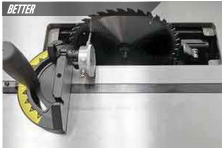
A dial indicator on a mitre gauge.
