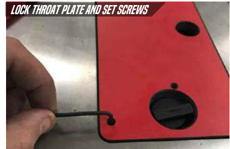
LOCK THROAT PLATE AND SET SCREWS Lock the throat plate in position and screw in the Alan set screws so that the table tries to force away and comes in contact with the locking mechanism. This will ensure that the throat plate will not move and stays in the same location during the next steps.
