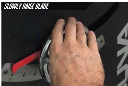
Give power to the table saw and SLOWLY raise the blade through the new throat plate. NOTICE: Use a respirator! Cutting the throatplate may contain particles that are harmful to the human body.
