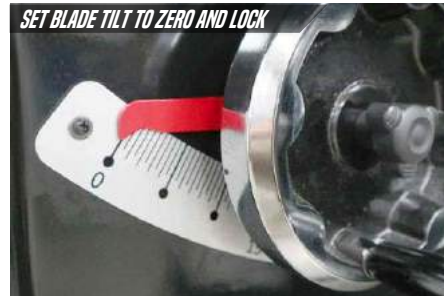
WARNING: MAKE SURE SAW IS UNPLUGGED. With the saw unplugged, set the arbor tilt to 0 degrees and lock the arbor tilt mechanism so it cannot move. It is wise to double check that the blade is 90 degrees to the table if this is a new saw. Set arbor height to lowest position and install new throat plate.
