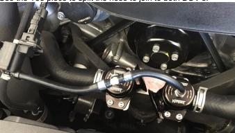
Congratulations, your Turbosmart Kompact Series BOV is installed and ready for use. Double check all connections and mounting screws. Start your engine and check for leaks.
