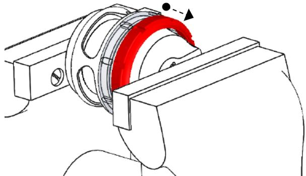
Inspect for Damage before inserting piston assembly into Raceport Body. Ensure Diaphragm bead is seated correctly in the groove on the body.
