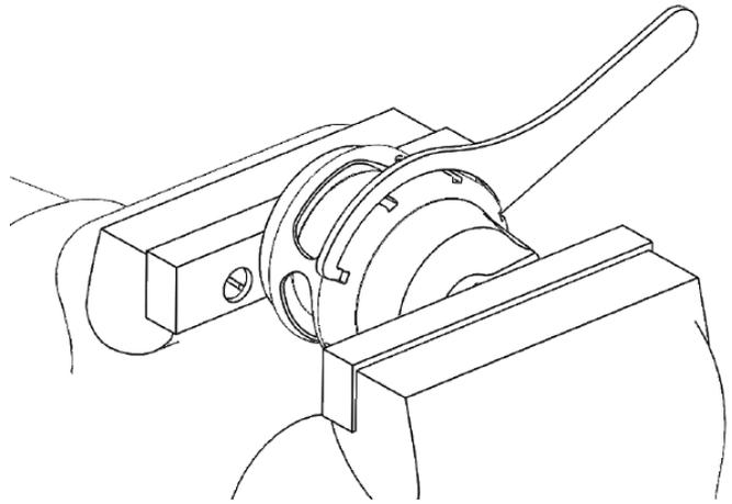
Reinstall fittings to the cap of the Raceport using fresh Loctite 567 thread sealant.
