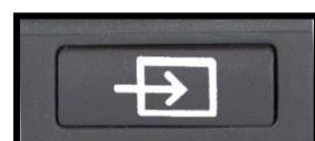
If a computer or another external source is connected to the ClearView C, press the grey PC button marked with an arrow (second button from the right) to toggle between the ClearView C image and the full screen computer image.
