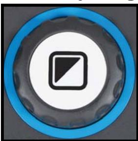
Pressing the white Mode button for four seconds turns off the object lighting. You may want to temporarily turn off the object lighting to eliminate light reflections. If you press this button again, you will continue to the next reading mode and the lights will turn back on. Pressing the button for four seconds will turn the object lighting back on but will not advance to the next reading mode.
