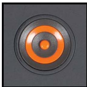
To power on both the system and monitor, press the orange round On / Off button located next to the Zoom dial on the Control Pad. The ClearView C will start up in the same viewing mode as when it was powered off.
