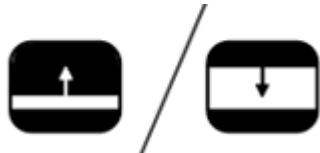
When line markers or window shades are activated, press the grey Lines / Windows button for 3 seconds. The top or left line or window shade blinks to indicate it can be moved up, down, left and / or right. Use the Zoom dial to move the line marker or window shade. Press the Lines / Windows button to adjust the other line or window shade. To move the other line marker or window shade use the Zoom dial. Press the Lines / Windows button again to exit Lines / Windows modification mode.
