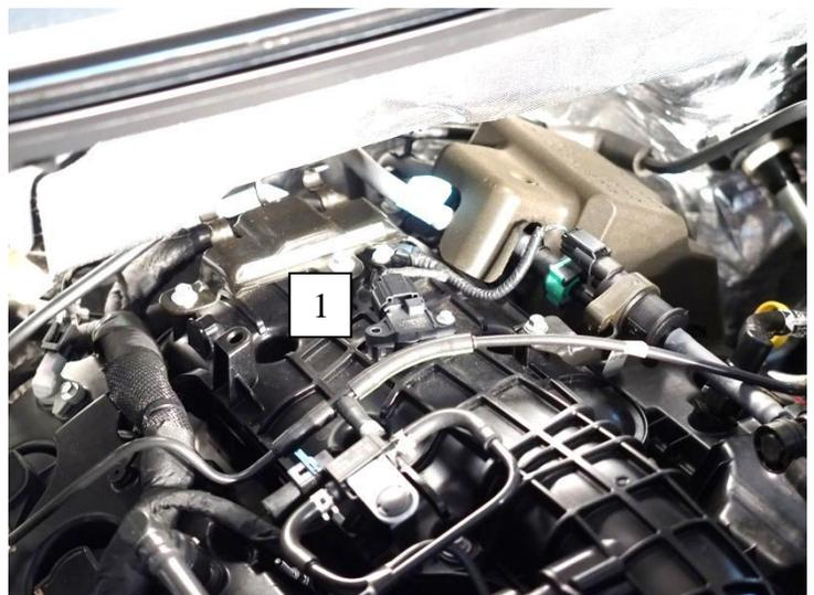
2. Install the supplied 1/8" NPT nipple on the MAP adapter. Blank off the second port on the MAP adapter if it is not in use. **Use thread sealant. Route the supplied vacuum hose from the nipple towards the front right hand side of the vehicle (OEM BOV location). Use one of the supplied spring clamps to secure the vacuum hose onto the nipple.**
