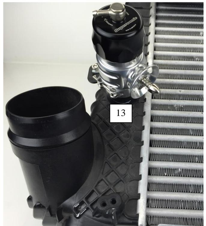
14. The finished intercooler assembly should look as shown on the right. Please ensure that all fasteners are secured prior to reinstalling the intercooler.
