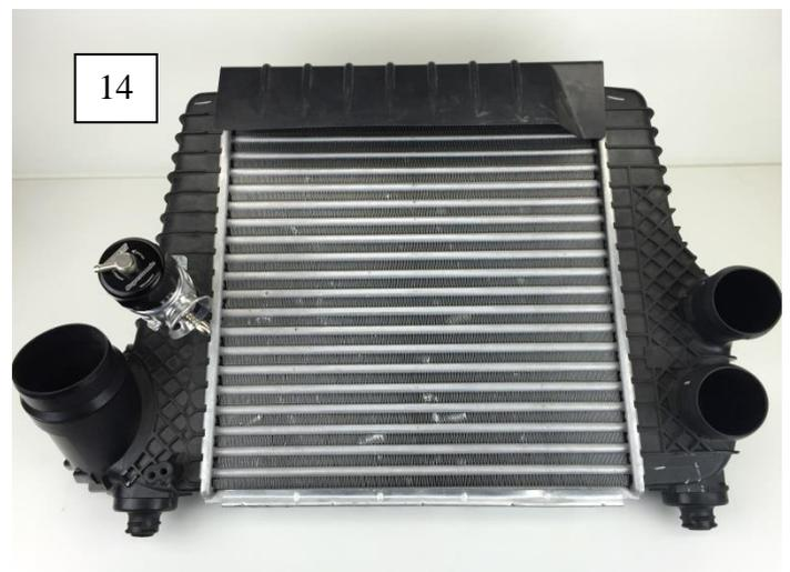
15. Prior to re-installing the intercooler back onto the vehicle. The OEM BOV plug needs to be blanked off. Depending on the purchased kit, you may receive either a direct plug-in plug option or a plug utilising scotch lock connectors. The direct plug-in blanking plug fits only one way. After blanking off the OEM BOV plug, secure it by using the supplied cable ties.
