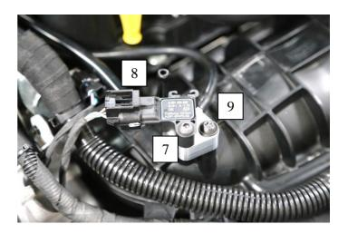
Route the vacuum hose towards the bottom rear left hand side of the engine towards the factory BPV location. (Bottom left hand side of engine when facing the vehicle.)
