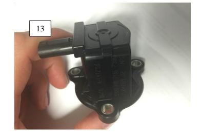
14. Install your new Turbosmart BOV. Align the mounting holes with the flange. Use the OEM M6 bolts to secure the BOV. Do not over tighten. Connect the vacuum hose (routed from the MAP adapter in step 9). Use the supplied spring clamps to secure the vacuum hose onto the BOV nipple.
