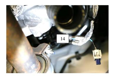
The OEM BPV solenoid plug needs to be blanked off. Depending on the kit purchased you may either be supplied with a direct plug-in blanking plug or a plug utilising clip-on connectors.
