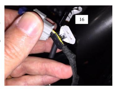
17. The clip-on connectors should look like this when installed correctly. Clip-on connectors are removable if the factory BOV is to be reinstalled. Secure the blanking plug with the supplied cable ties.
