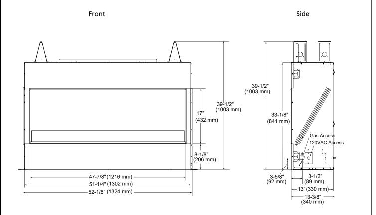
3" minimum under appliance. 6" minimum under appliance with optional drain pan (ODLANAIG-48DP)
