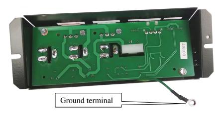
For newer NGX cabinets with a ground stud just below the Power Distribution Unit, connect the ring terminal to this stud reusing the #8-32 hex nut. Be sure the wire is not pinched by the chassis during installation.
