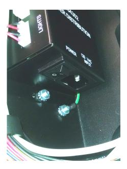
For older NGX cabinets without a ground stud in the cabinet, connect the ring terminal to the screw holding the circuit board as shown here before installing the unit in the NGX cabinet.
