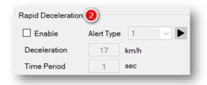
**Note:** For example, if the Speed threshold is set to 20 km/h and the Seconds value is 1, an event occurs if the vehicle reduces speed by more than 20 km/h in one second.
