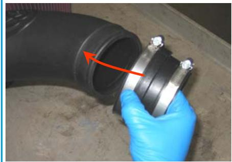
**3.** Loosen the hose clamps at the OE air box and at the turbo inlet, then remove the OE intake tube.
