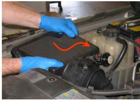
**9.** Place the S&B Air Box assembly into the vehicle, align the 4 holes with the OE mounting locations and secure using either the OE bolts or the supplied hardware. You may need to loosen these bolts to align the tubes during step # 12, then retighten.
