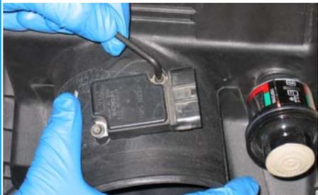
15. Peel the backing from the MAF Sensor Gasket (H) before placing it over the sensor, sticky side down.
