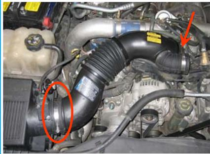
**7.** Remove the OE air box tray. If long enough, you may use four of these bolts to secure the S&B Air Box (D) to the vehicle. If not use the supplied M6 allen head screws (R) and SS washers (S).
