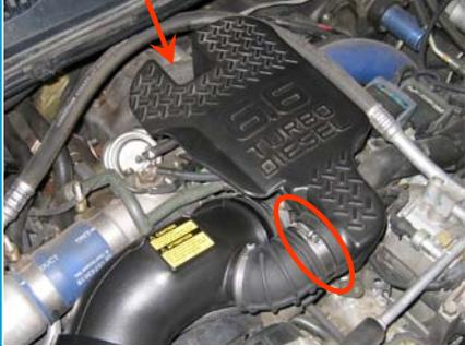
**6.** Remove the OE foil from the inner fender, this will allow cooler air to enter the S&B air box.
