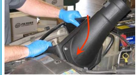
**2.** Loosen the bolt and the hose clamp that secure the OE resonator chamber and remove the chamber from the intake tube.
