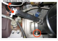
5. Loosen the hose clamp on the intake tube to assist with the removal of the air box.
