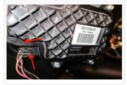
9. Once the sensor is disconnected, completely remove the factory air box and intake tube by lifting up and out.
