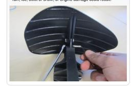
16. Install the provided Inlets (G&J) and Tube Seal (Q) into the Air Box (I) by inserting and snapping into place. A bit of force and effort may be necessary to install inlets and seal. Line up each part with the dot on the box.
