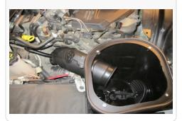
23. Install the Hose (T) with #16 Hose Clamp (Y). Next install Silicon Adapter (Z) and #64 Hose Clamp (AA) onto the Intake Tube (X). Remember to only tighten Hose Clamps (Y) and (AA) on the tube side.
