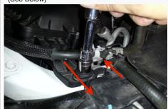
7. Lift up on factory air box, be careful not to remove the whole box because the swing gate motor harness is still connected on the side of the air box. Remember to move the hose forward from Step 6 when pulling out the box.
