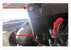
24.(b) Reach under the air box to feel if the posts pushed through the holes (grommets). Be careful not to push to hard or the tabs will break off the battery tray.
