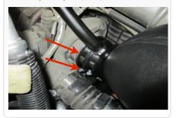
28. Install the Hose (CC) onto the crankcase ventilation line.
