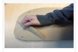
33. Install the provided Edge Trim (C) around the lid. Once edge trim is installed roll the sides of the lid on a flat surface to ensure a tight seal. Once edge trim is installed roll the sides of the lid on a flat surface to ensure a tight seal.
