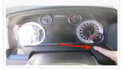
D. Carefully drill a hole using a 5/16" drill bit, use lower rpm speeds and start hole with smaller bits
