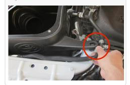
**26.** Push down on air box and tighten the provided Retaining Bolt (H). If the bolt does not align correctly please go back to step 36 to make sure the box is set correctly.
