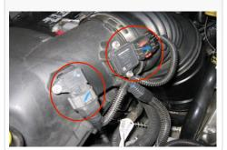
3. For the MAF sensor, slide the red locking tab up then depress the black lever while disengaging the connector. For the IAT sensor just depress the grey lever while disengaging the connector.
