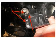
18. Note: Do NOT remove Swing Gate Arm (S) after installing it to the motor as this could damage the snap in feature of the arm. If removal of Swing Gate Dam (N) is desired, remove with Swing Gate Arm (S) installed on Factory Swing Gate Motor (L).
