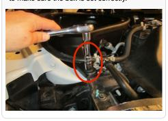
27. Connect Silicon Adapter (Z) to turbo and tighten #64 Hose Clamp (AA). Please make sure the coupler is push all the way onto turbo before tightening completely.
