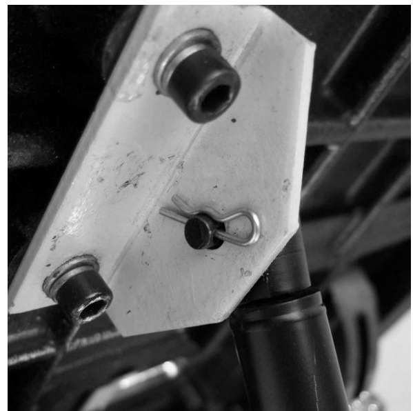
Gas assistor fitted to table
