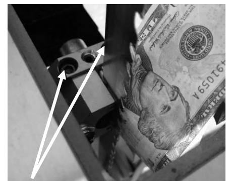
Forward & back clamp screws
