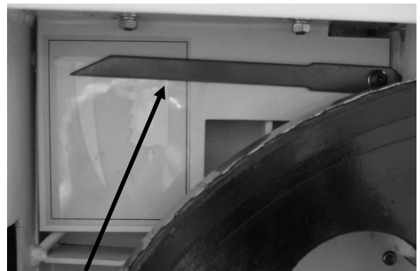
Blade tension indicator
