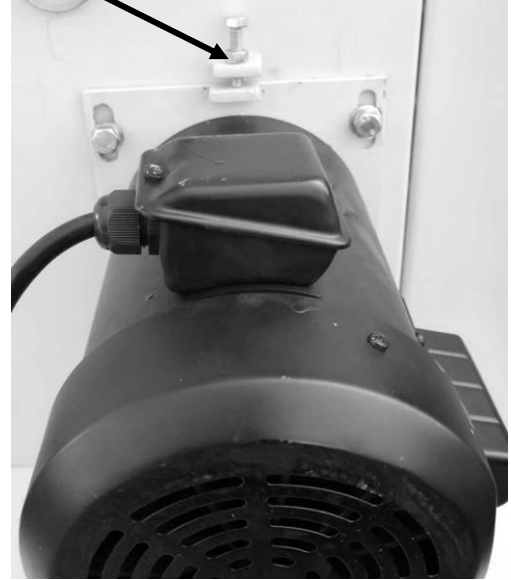
Belt tensioning bolt
