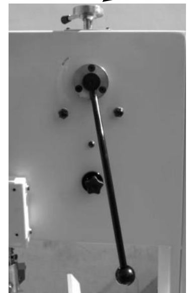
Blade tension hand wheel
