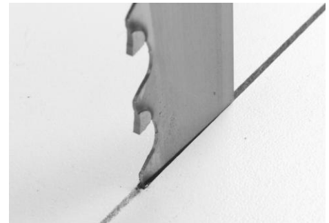
Blade not centered in saw cut
