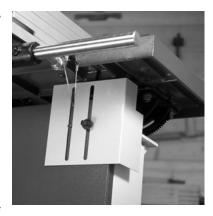
Align the guard on the bolt and install the thumbscrew on the outside of the door.
