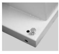
head, the door will not be able to be opened. **5.** Adjust the bolts so that the machine is level in both planes and does not rock.
