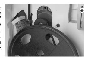
A brush contacts the lower wheel and helps to prevent buildup. You should inspect the tires regularly to check that buildup is not happening, especially the lower wheel. The tires are made of rubber and wear just like car tires. They wear in the middle, which causes a concavity in the tire. The deformation makes it hard to track the blades, and for this reason it is important to maintain the original shape of the tire.
