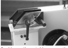
Position the table on the trunnion, taking care not to damage any of the table or trunnion surfaces.
