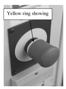
Stop switch in the on/out position (should see yellow ring)
