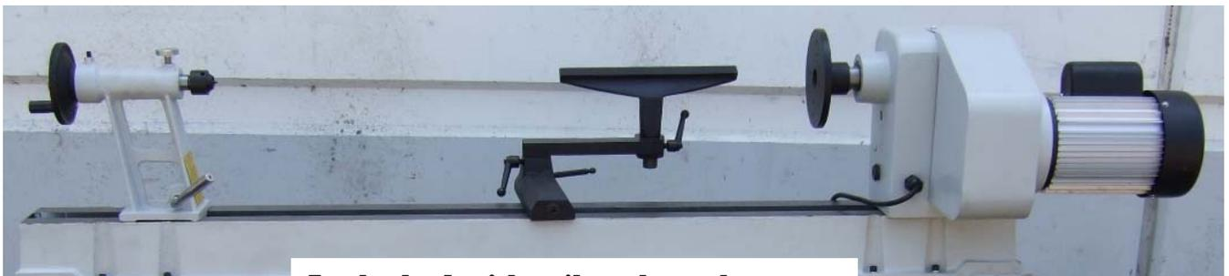
**Lathe bed with tailstock, tool rest, and headstock assembled**
