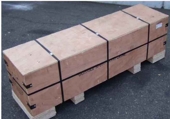
2. Dismantle the box, including the sides as this will ease access to the machine.
