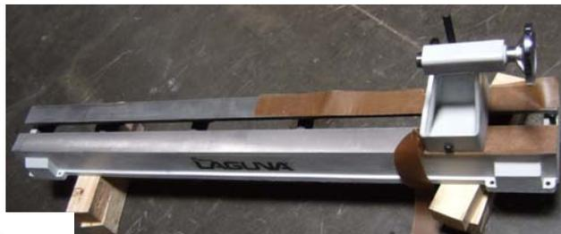
**Lathe bed shown with the head stock removed.**
