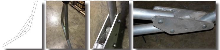
1. Locate corner frames shown above. Mount each side to mounting bracket on front of 'V' shaped lower frame assembly. Also secure V frame to already welded front bracket as well. Use 3.5"L bolts and nuts and washers provided in hardware bag (Part G).
