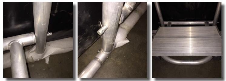
1. Install pre-assembled coach's platforms on each side of dolly assembly by inserting long rod through back frame assembly and inside shaft of coach's platform as shown in pictures above. Secure with heavy duty cotter pins.
