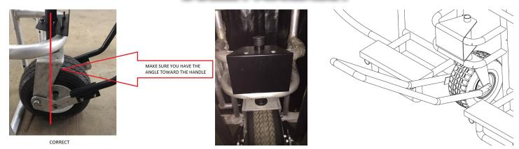
1. Attach dolley assembly mounting plates as shown in pictures above. Be sure black mounting shaft is attached to plate as shown using proper ring spacer between tire mounting plate and shaft.
