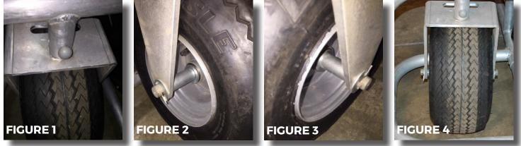
1. Locate (2) turf tires and mounting plate shown in illustration above. Hardware for the wheel assembly is located in bag 'Part I'. Wheel shafts are located in 'Part J'.
