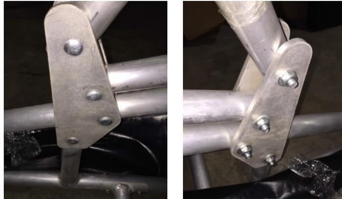
1. Using same bolts, nuts, and washers from Step 6 above, attach angle bracket to 'V' shape lower frame. The bracket will attach midway up the frame on holes provided.
