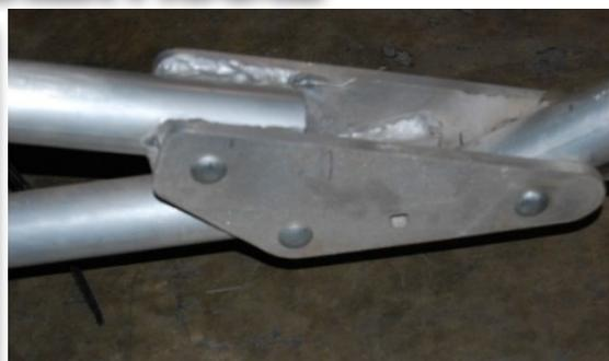
1. Locate corner frames shown above. Mount each side to mounting bracket on front of 'V' shaped lower frame assembly. Also secure V frame to already welded front bracket as well. Use 3.5" L bolts and nuts and washers provided in hardware bag (Part G).
