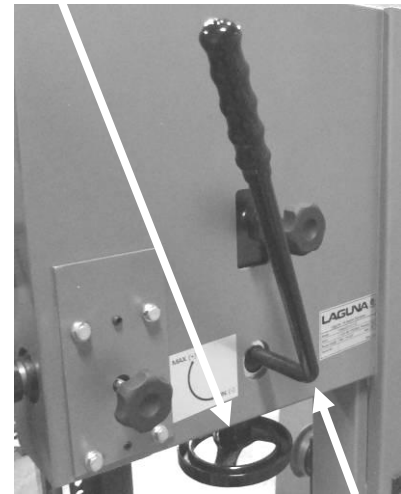
Quick action blade tension lever (activated)
