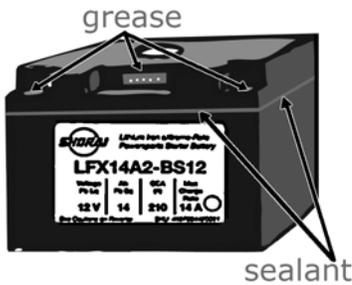
**WATER/CORROSION:** Avoid high pressure power washing around the battery case, or constant exposure to water. If the battery may be occasionally submerged, we highly suggest application of sealant to **fill the horizontal seam between top and bottom of the battery case**, and that the 5-pin port be fully packed with **dielectric grease**. (dielectric grease is a good idea in any case to insure no pin corrosion). Also, heavy grease should be liberally applied to terminals for wet environments.
