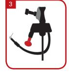
The Lock-N-Load harness line will then disconnect and free the harness spreader bar and rider from the Lock-N-Load safety system.
