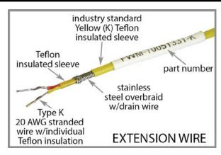
The Type K, 20 AWG stranded extension wire encased in a rugged cable meets demanding environments. The industry standard yellow Teflon allows easy identification of K type thermocouple wires so they can be separated from high voltage wires following good installation practices.
