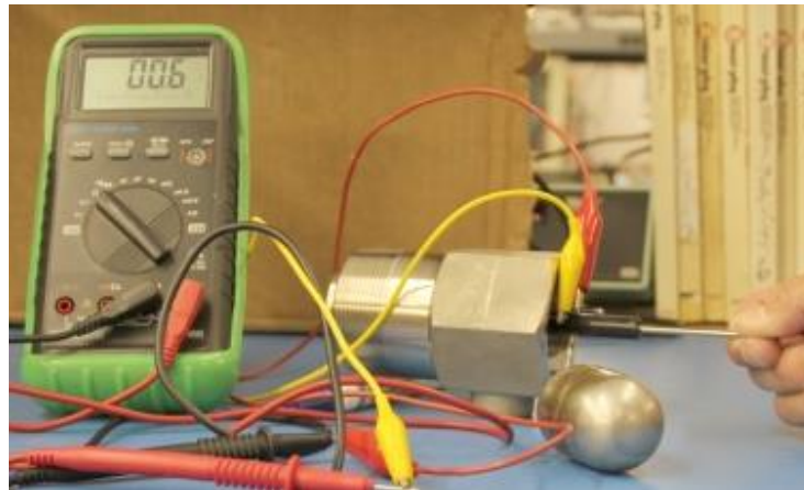
Figure #2 Float is Missing
