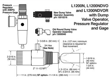
Note: For use only with Old Round Dump Valve Operator Assembly (15000940).
